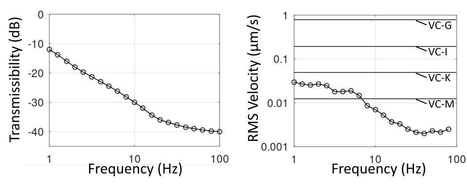
Measured with Wilcoxon 731A in one-third octave bands according to ANSI S1.11-2014 standard
